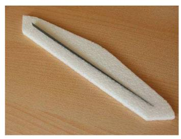
Fixed part of elevator cut across and add carbon tape  $8x\ 0.3\ mm$ .
