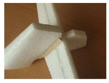
Stick reinforcements from balzy triangular cross section.
