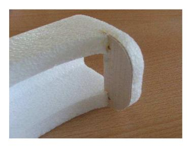
For sealing the front portion of plywood make slit in the hull.
