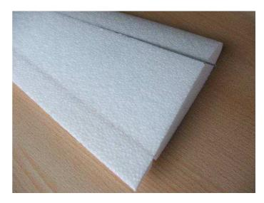
A sharp knife cut a groove to insert a carbon tape. Belt have to exceed in the middle of the wings about 10 mm.
