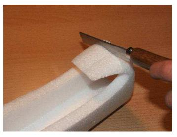
Cut off the buttom of the mddle part of fuselage.
