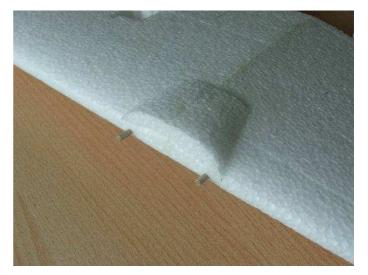
Glue up two wooden pegs. At the middle bottom of the wings stick cutting of part of the hull.
