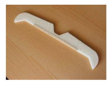
On the floating part of the elevator stick reinforcements from balsa  $8x4\,$  mm
