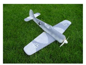
In the end, check the position of the centre of gravity. In case heavier motor is mounted, make weight balancing in the rear part. Set rudder deflection to  $30^{\circ}$  at the beginning. It is recommended to make first test flights during windless weather.
