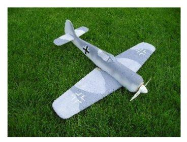
In the end, check the position of the centre of gravity. In case heavier motor is mounted, make weight balancing in the rear part. Set rudder deflection to  $30^{\circ}$  at the beginning. It is recommended to make first test flights during windless weather.
