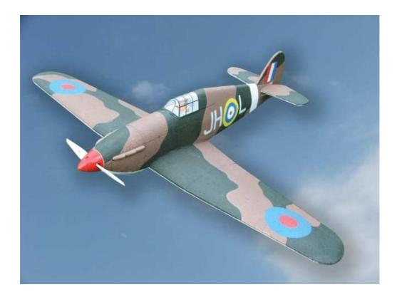
In the end, check the position of the centre of gravity. In case heavier motor is mounted, make weight balancing in the rear part. Set rudder deflection to 30° at the beginning. It is recommended to make first test flights during windless weather. Always fly in such a way to avoid injury to yourself as well as to your surroundings.
