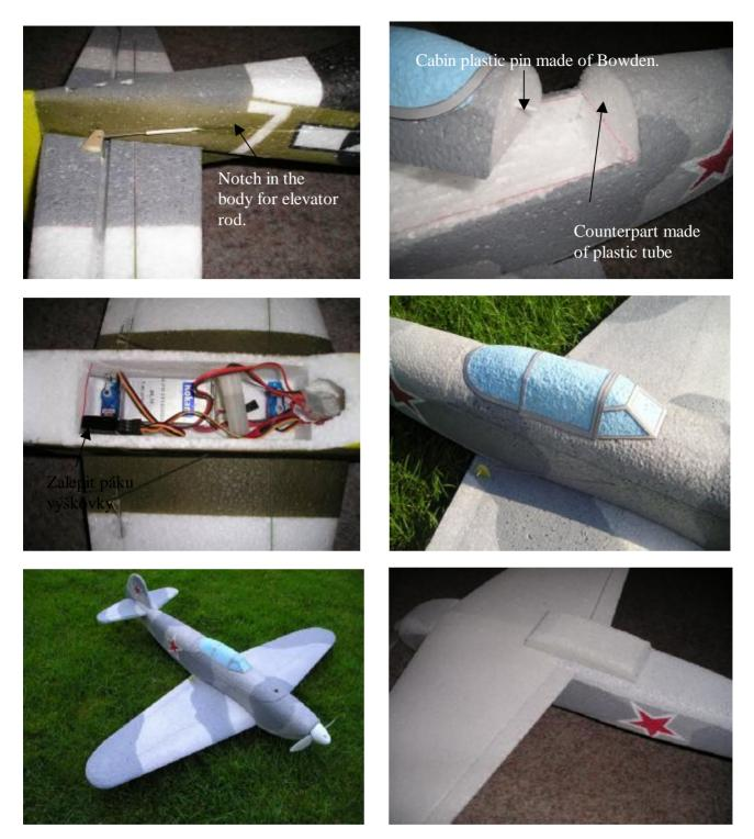
In the end, check the position of centre of gravity. In case heavier motor is mounted, make weight balancing in the rear part. Set rudder deflection to  $30^{\circ}$  at the beginning. It is recommended to make first test flights during windless weather.
