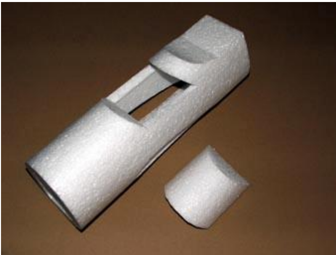
9) Cut the removeable cover, lower fuselage part
