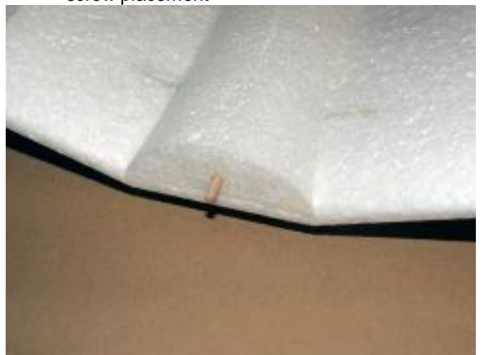
Glue the rear plywood part for plastic female screw placement
