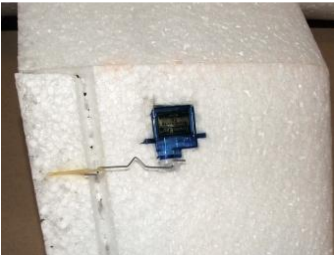
21) Push rods made up from iron wire
