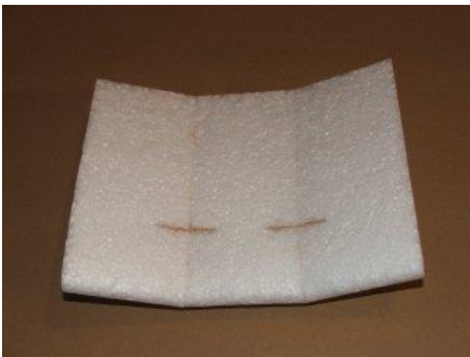
5) Glue center and inner wing sections together
