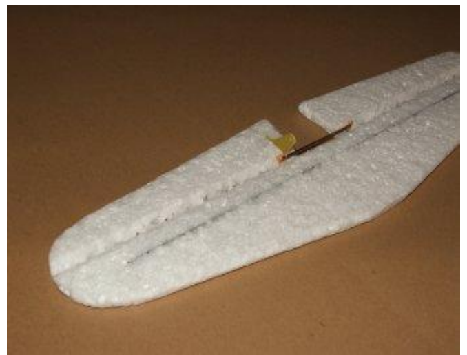
18) Join the elevator using U-shaped iron wire. Glue the control crank into the cut
