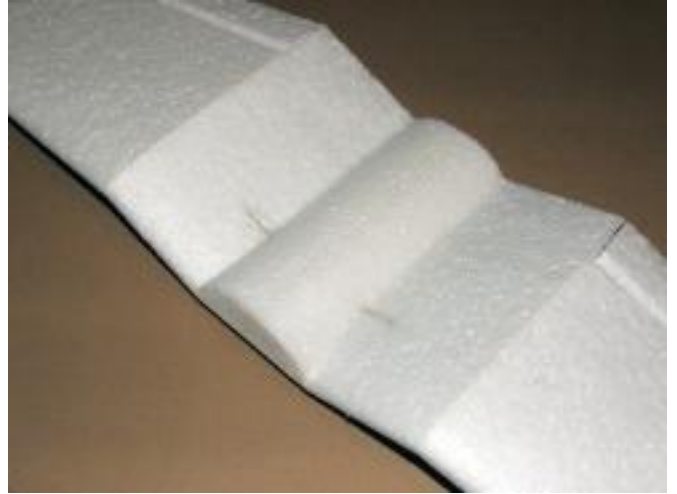
Glue the cutted part to the lower wing surface
