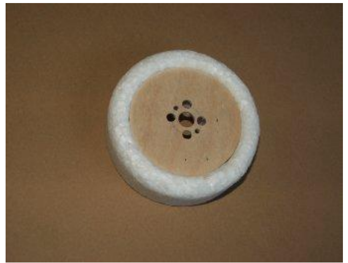
14) Drill engine mounting holes and glue the engine bulkhead
