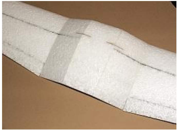
8) Glue the wing sections together
