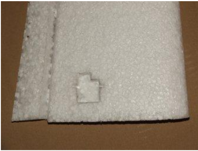
1) Cut the servo compartment
