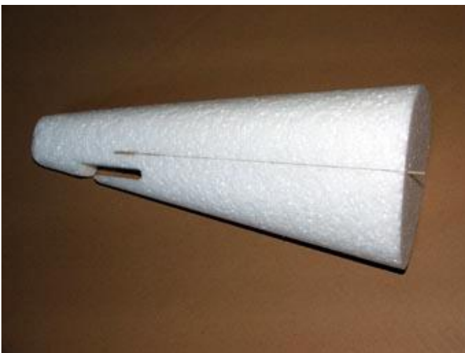
11) Make the cut for bowden, rear fuselage part
