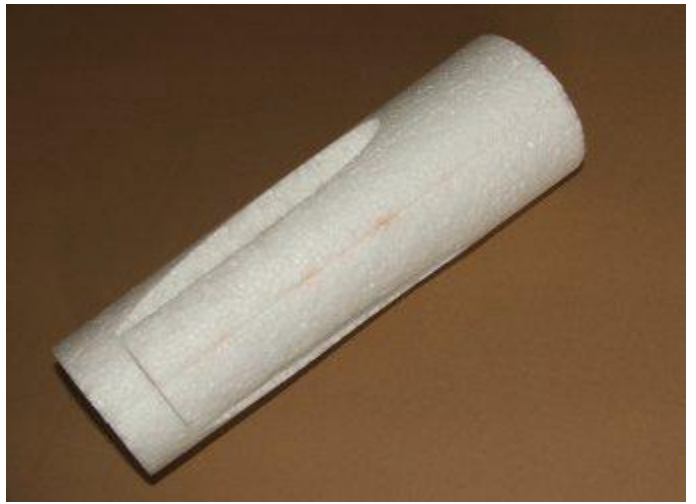
10) Glue the cross-cutted lower fuselage part
