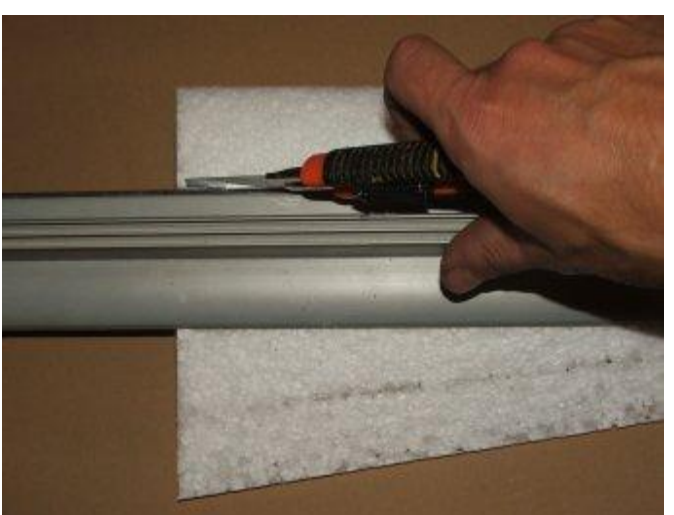
6) Make a cut for carbon stripe using sharp knife
