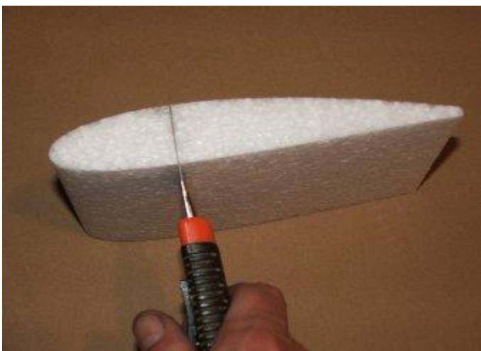
3) Make cut for wing plywood joint
