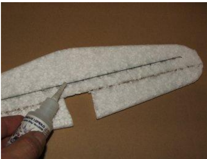
17) Make a cut and glue the carbon stripe
