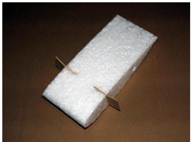
4) Glue the plywood wing joints to the center part
