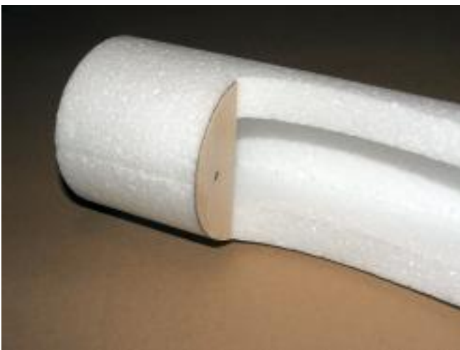
Glue the front plywood part
