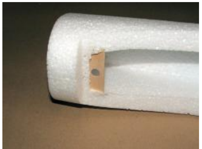
Glue the rear plywood part for plastic female screw placement
