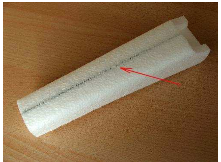
In the bottom glue carbon reinforcement strip
