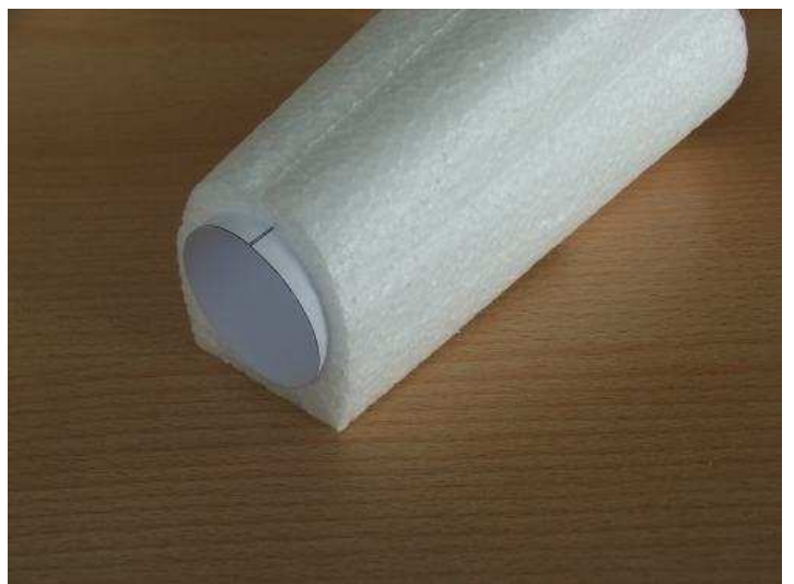
Paper tube insert and stick up to the rear of the fuselage
