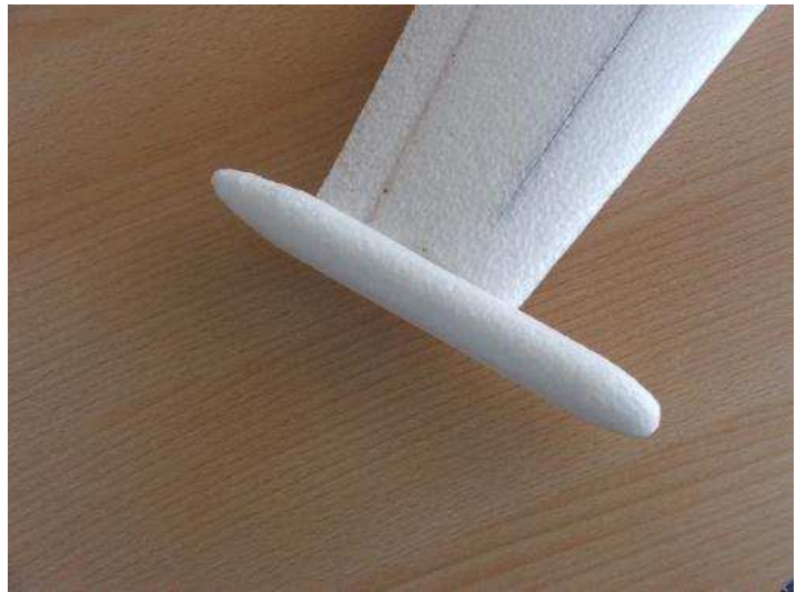
At the end of the wings attach "additional tanks"
