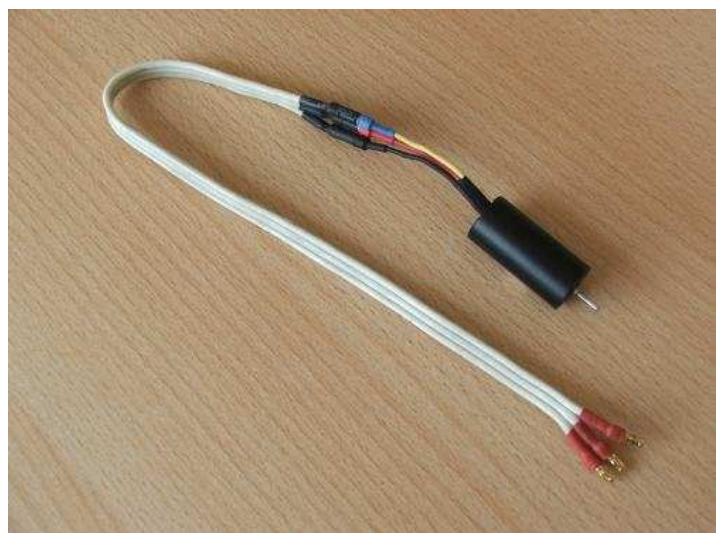
Prepare an extension cable for motor
