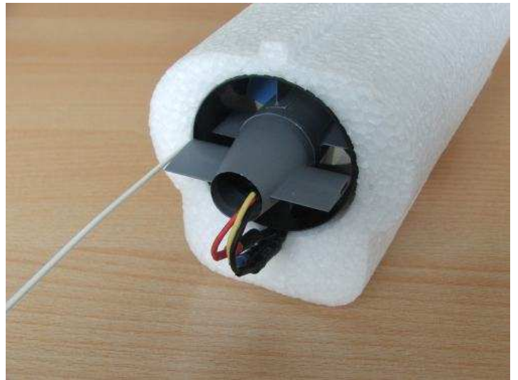
Blower together with the engine installed in the central part of the fuselage.
